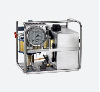
To stand up to tough offshore environments, HYTORC has taken our tried and true high flow pneumatic pump and reconstructed it with stainless steel components. Additionally, we have doubled the size of the reservoir to suit the demands of subsea fastening.
