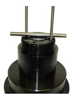
Screw the Piston fully into the Nut Body.
