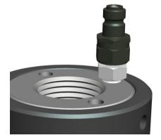
Using a spanner, firmly tighten then the nipple or coupling onto the adaptor. Take care not to over tighten the adaptor into the Nut.
