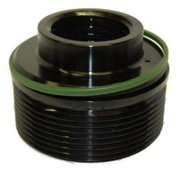
Stretch the seal over the outer lip of the piston by working around both sides of the piston simultaneously.
