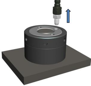
The Hydraulic Nut can be unscrewed.
