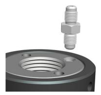
Check the internal and external threads are clean and free from damage.
