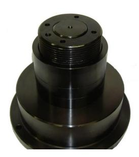
The Piston is fitted and the nut is ready to receive the Load Retaining Collar
