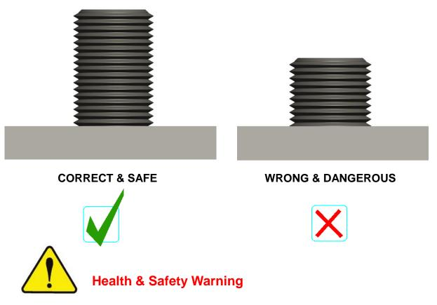
If insufficient threads are engaged at either end of the bolt, and an attempt is made to apply tension with the hydraulic nut, the bolt or nut threads may strip and components of the nut and or the bolt, could be launched with the possibility of serious injury.
