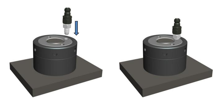
Connect the hydraulic hose. Make sure the quick connect coupling is fully engaged.
