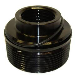
Place the Piston on a clean surface. Insert the rubber "O" ring into the seal groove.
